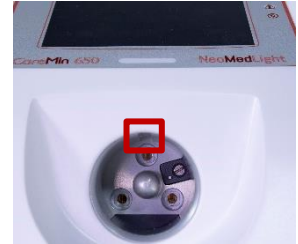
Figure 4 Connector insertion: the mistake proofing slot (left picture) should be set onto the fence (right picture)
